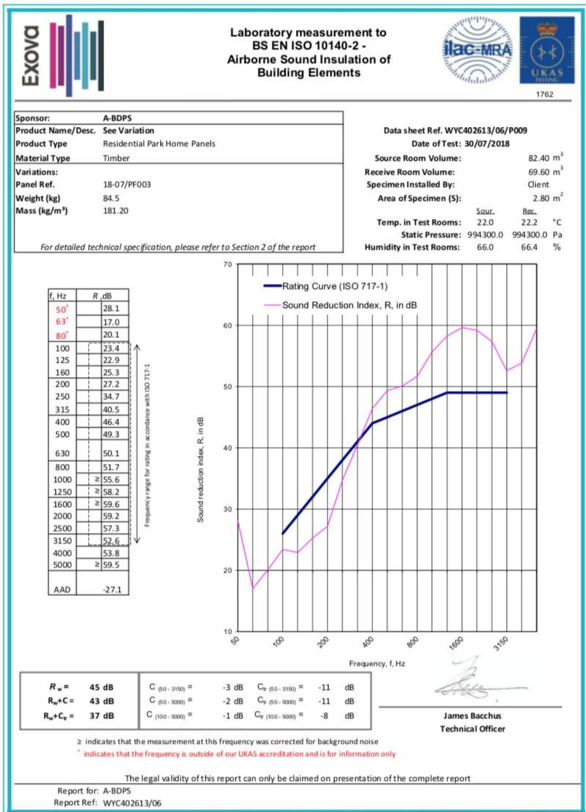
Figure 10. Example of Enhanced Rw45dB Mobile Home External Wall Test Result Graph
