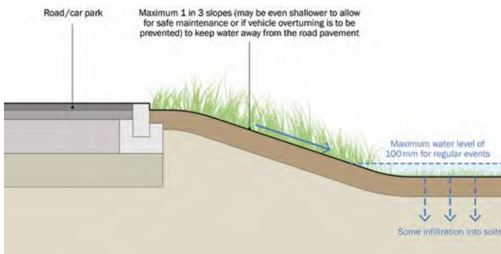
Figure 9.13 Water flows from shallow swales acting as edge drains for the road sub-base
